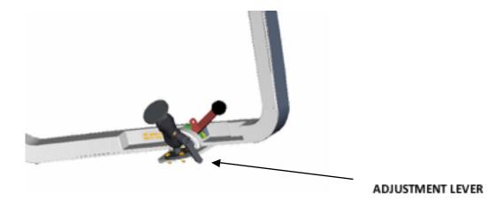
FIGURE 1: Captain's Side Window Modified with EZ Mount Arm (First Officer's Installation is Mirror Image)
