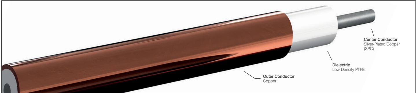
Low-loss semi-rigid cables provide lower attenuation, better phase stability with temperature, and a higher operating temperature compared to traditional solid PTFE semi-rigid cables.
