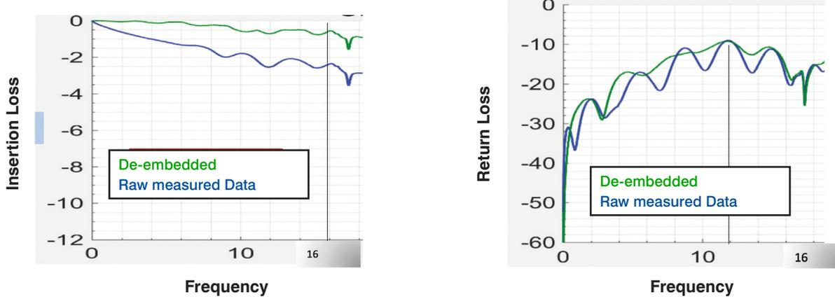
Fig. 44: Insertion and return loss of the Card Edge Connector system
