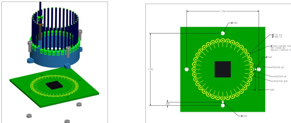
Fig. 24: Vertical-mount CoreHC interconnect with custom housing
