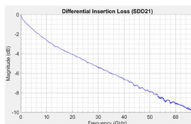
Fig. 10: Differential insertion loss of a CoreHC interconnect using a .079-inch coax cable
