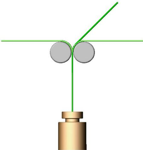
Fig. 5: Test setup for high-stress flex testing
