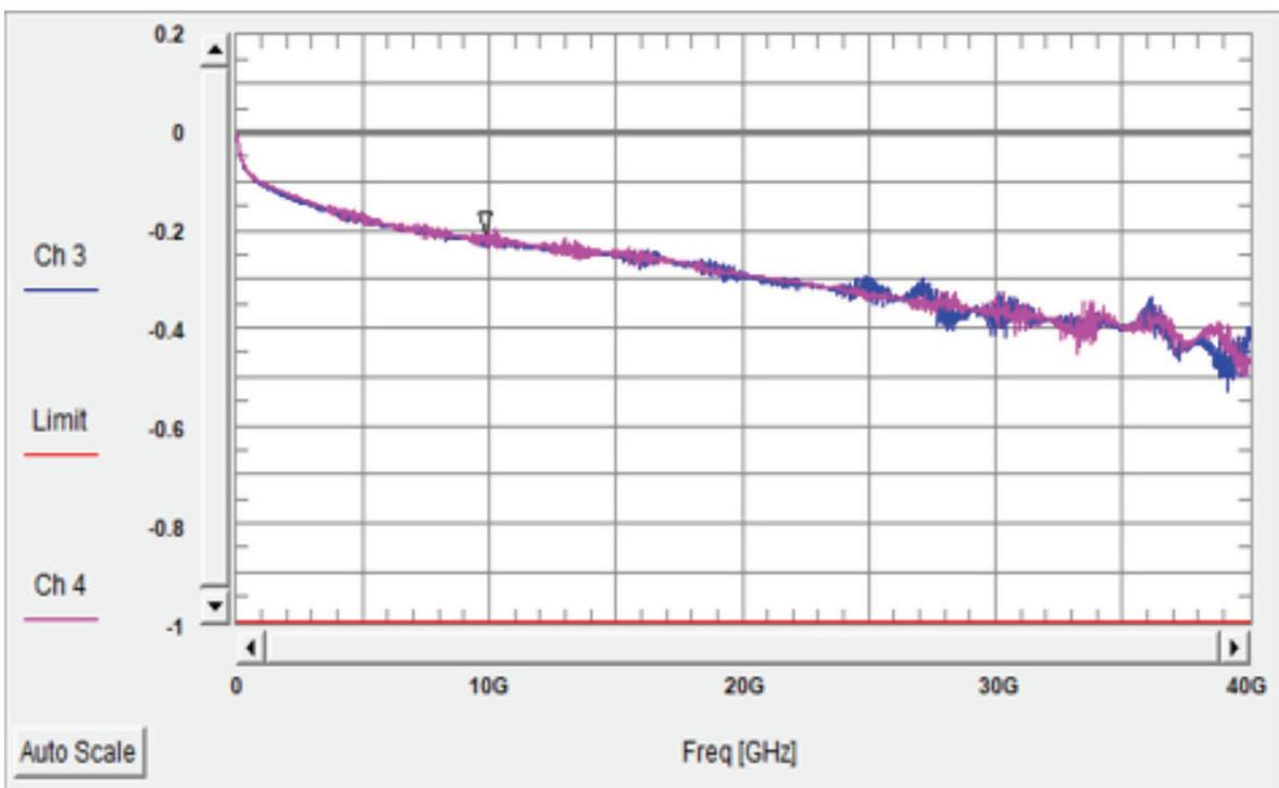
Fig. 39: Low insertion loss of a 2.92-mm female to 2.92-mm female adapter
