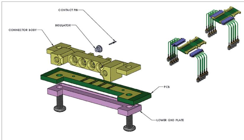
Fig. 24 (b): Edge Launch CoreGD Interconnect
