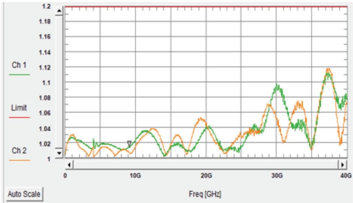
Fig. 38: VSWR performance of a 2.92-mm female to 2.92-mm female adapter
