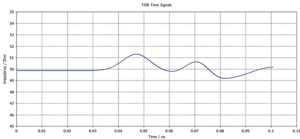
Fig. 33: Time domain response of a vertical-mount field-replaceable 2.92-mm connector
