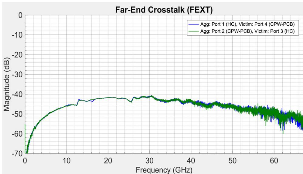
Fig. 18: Far-end crosstalk of the CoreHC interconnect and PCB in CPW PCB
