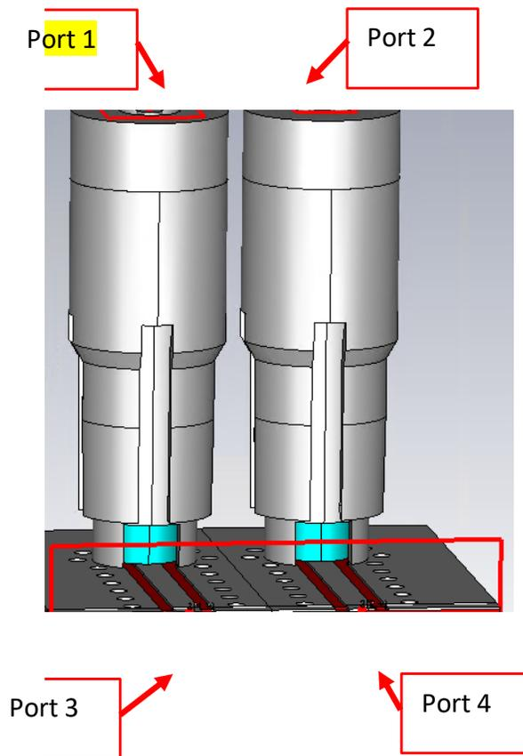
Fig. 16: Two-port CoreHC interconnect setup on a coplaner waveguide PCB
