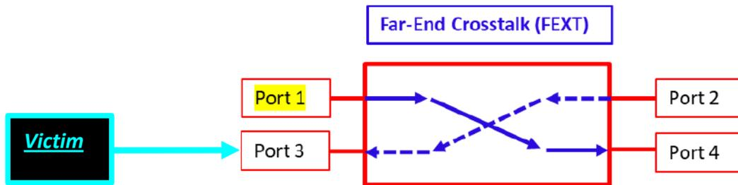
Fig. 15: Far-end crosstalk in two-port interconnect network
