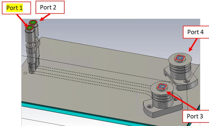
Fig. 19: Simulation setup of a two-port PCB with stripline traces using a CoreHC interconnect
