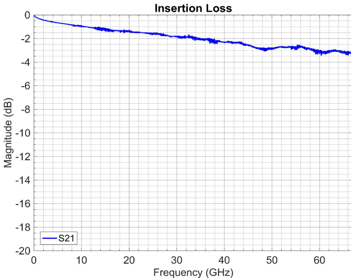
Fig. 2: Insertion loss of a .079-inch RF coax
