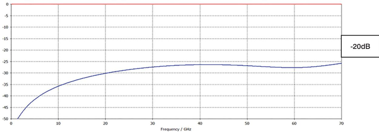
Fig. 32: Insertion loss and return loss of a vertical-mount field-replaceable 2.92-mm connector
