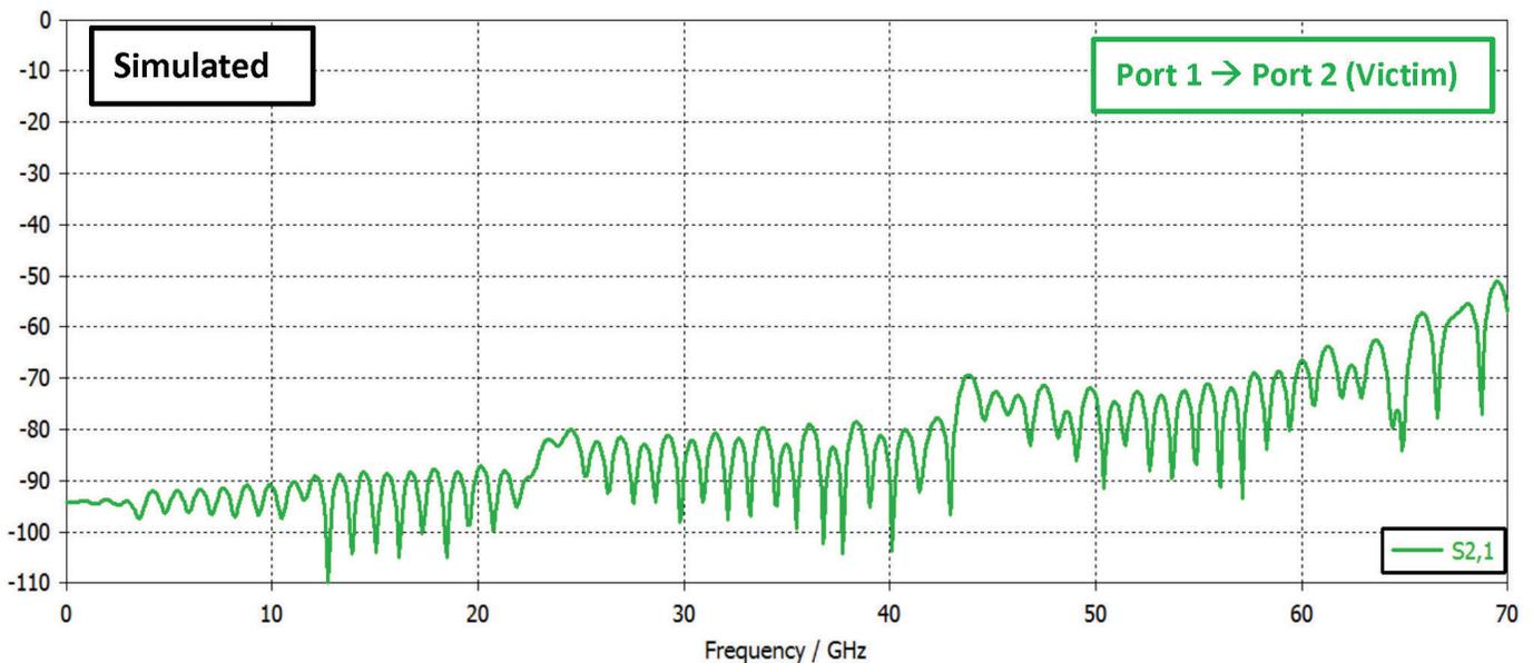
Fig. 20: Near-end crosstalk of a stripline PCB using a CoreHC interconnect
