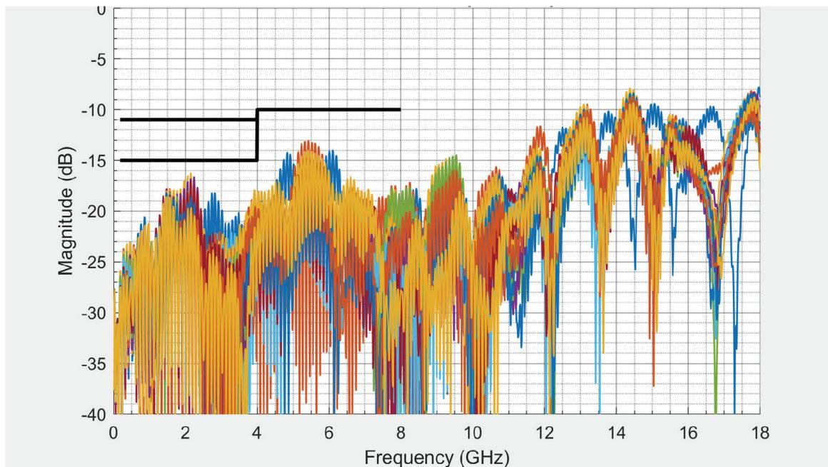
Fig. 47: Return loss of different channels in a card edge-based Twinax cable assembly
