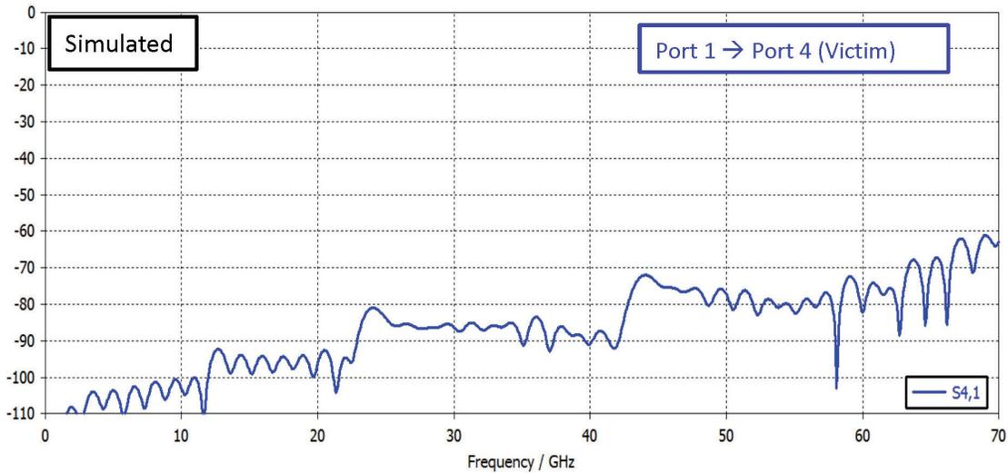
Fig. 21: Far-end crosstalk in a stripline PCB using a CoreHC interconnect
