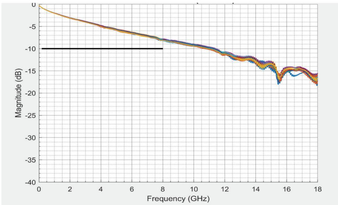
Fig. 45: Insertion loss of a card edge-based Twinax cable assembly
