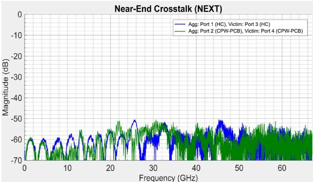
Fig. 17: Near-end crosstalk of the CoreHC interconnect and PCB in CPW PCB
