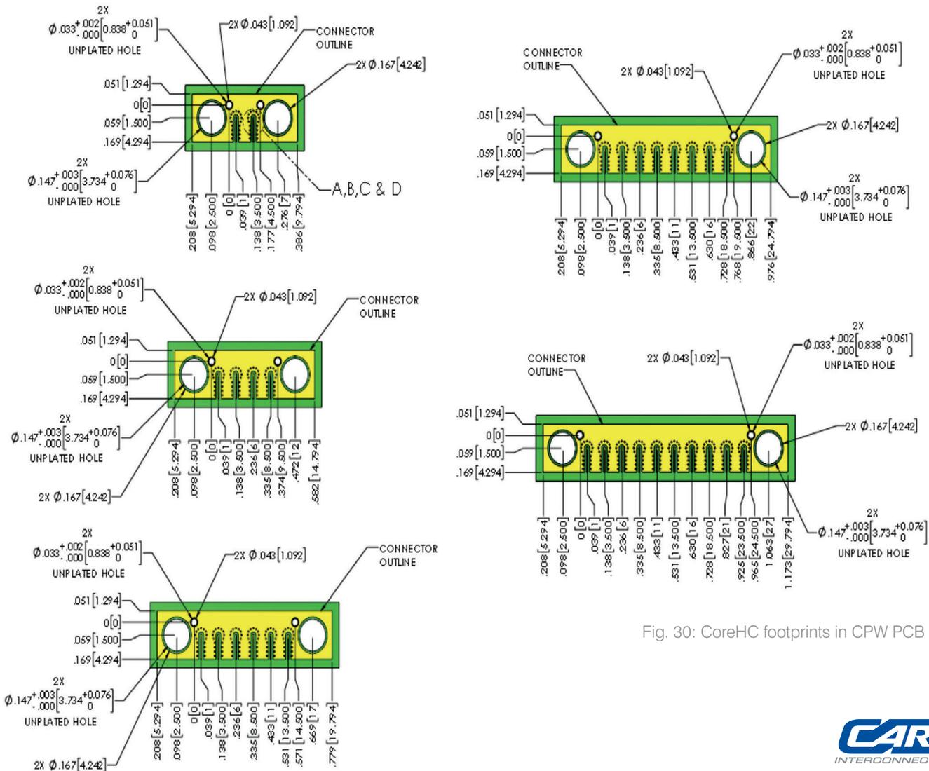
Fig. 30: CoreHC footprints in CPW PCB
