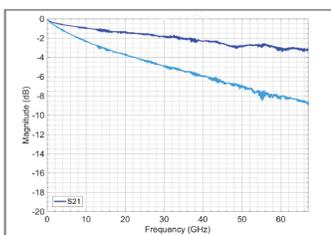
Fig. 9: Insertion loss of a 28 cm .079-inch coax CoreHC channel and cable assembly along with the trace
