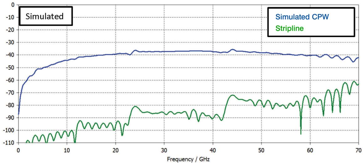
Fig. 23: Comparing far-end crosstalk of a CoreHC interconnect in stripline and CPW designs
