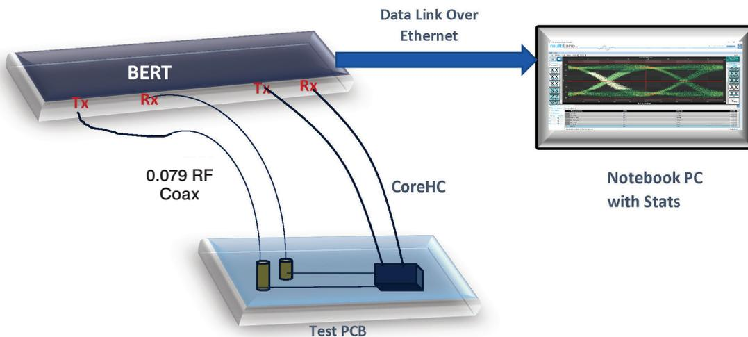
Fig. 27: Test setup using CoreHC, PCB, and .079-inch RF coax jumpers
