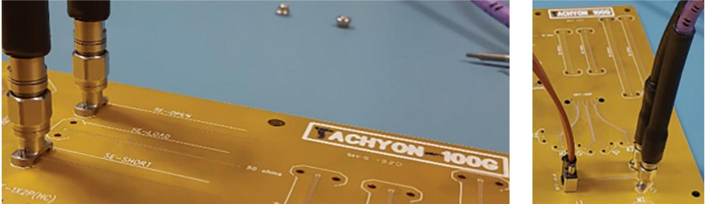
Fig. 13: CoreHC interconnect on a CPW PCB cross section
