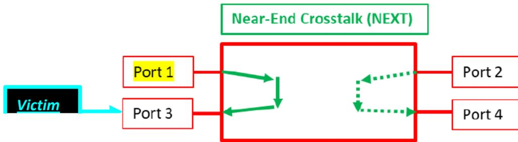
Fig. 14: Near-end crosstalk in two-port interconnect network
