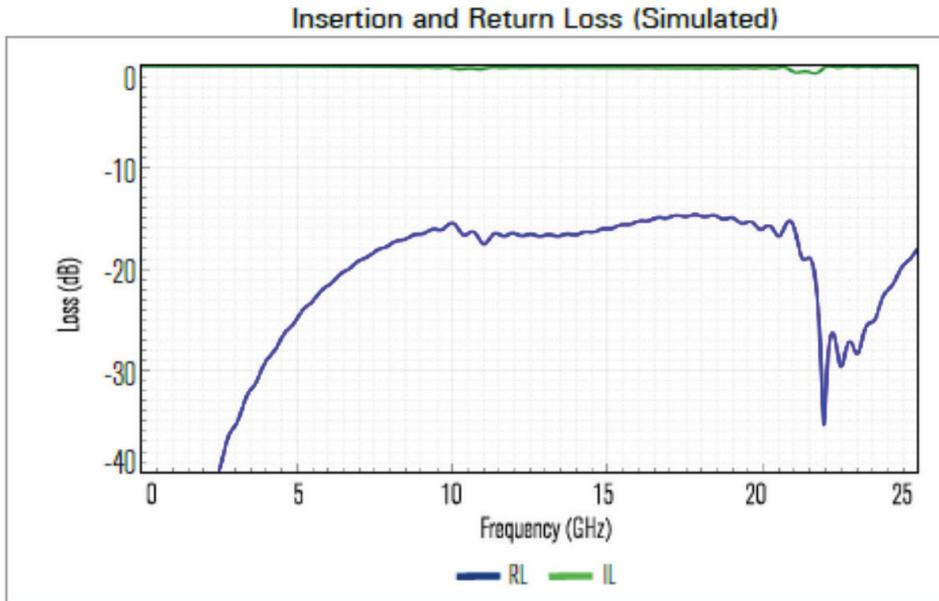
Fig. 42: Insertion loss and return loss performance of the AltaVel connector system
