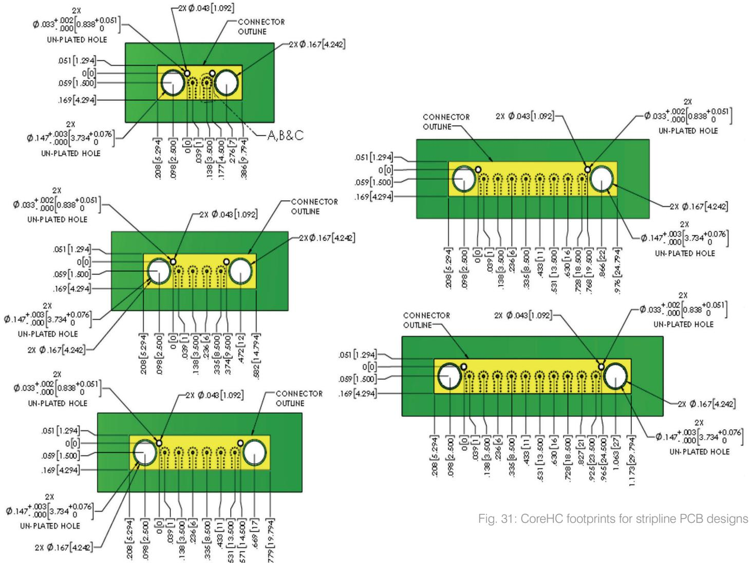
Fig. 31: CoreHC footprints for stripline PCB designs
