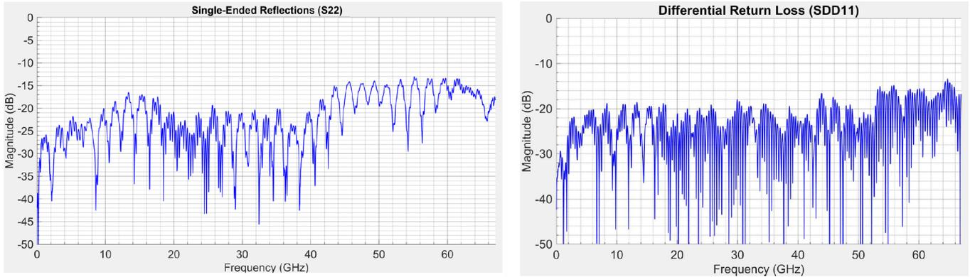
Fig. 11 (Left) and Fig. 12 (Right): Comparison of single-ended and differential return losses of the CoreHC assembly
