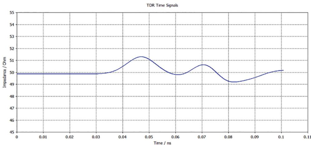
Fig. 35: Time domain response of a vertical-mount soldered 2.92-mm connector
