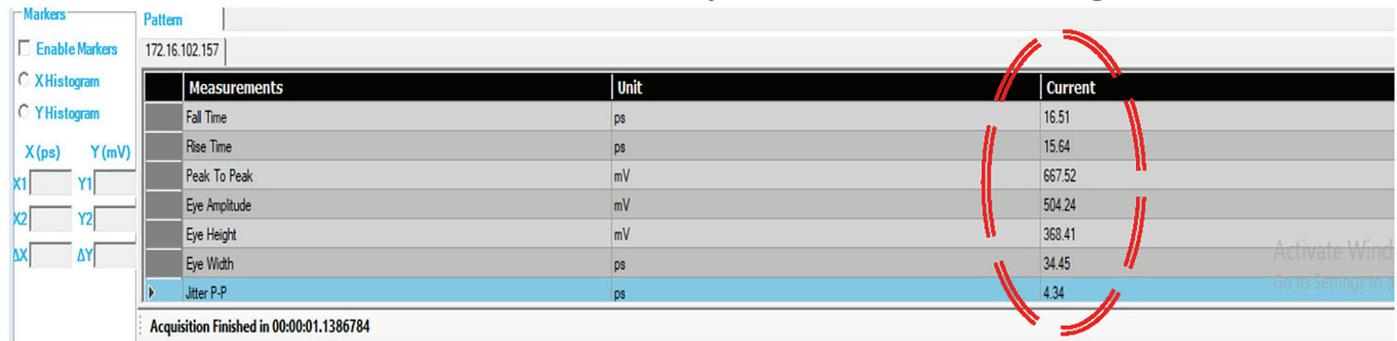
It can be concluded that the closing of the eye with the replacement of 6 inches of the coax cable section (in 1-foot test path) with a CoreHC cable assembly and PCB trace is almost negligible and does not affect the sampling of high-speed signals in electronic systems. Therefore, in a complex, highly-dense board layout, the coax cables can be replaced without the CoreHC interconnect time or frequency domain signal integrity concerns.
