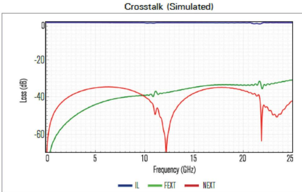
Fig. 43. Near-end and far-end crosstalk performance of a AltaVel system
