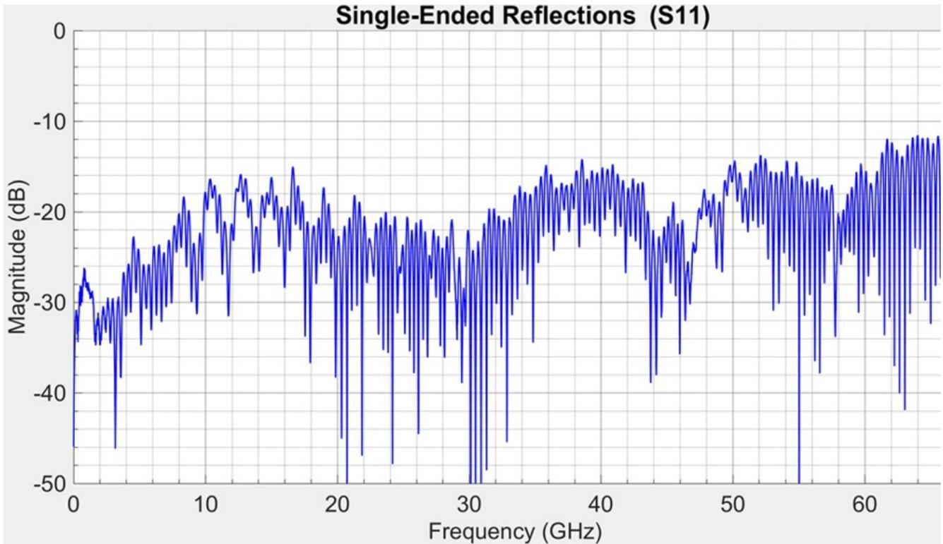
Fig. 3: Return loss of a 0.079-inch RF coax
