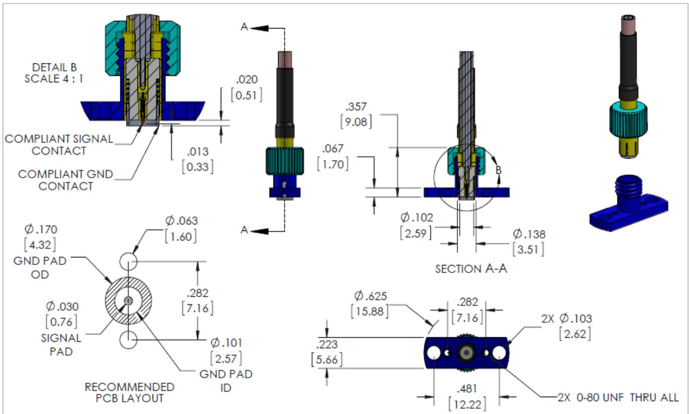
Fig. 25: Single-channel CoreHC-based secure interconnect solution
