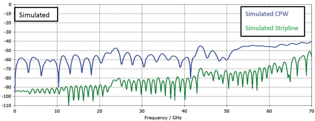
Fig. 22: Comparing near-end crosstalk of a CoreHC interconnect in stripline and CPW designs
