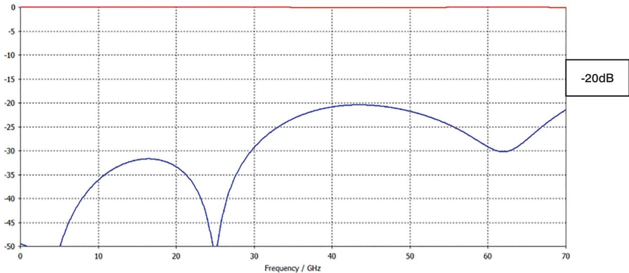
Fig. 34: Insertion loss and return loss of a vertical-mount soldered 2.92-mm connector
